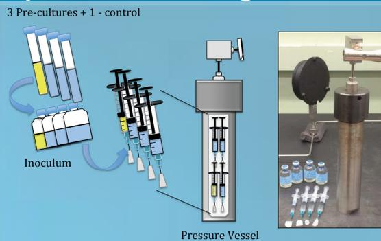
**Figure 2:** High-pressure batch culture procedure in 5 mL plastic syringes.
